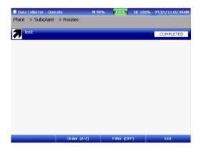
A measurement route is the grouping of multiple computers on a plant or a sub plant, sorted according to collection.
